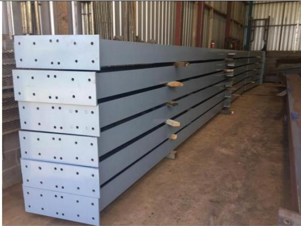
Image showing completed rafter to be transported to site.
