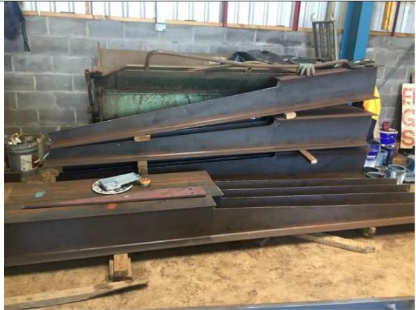
Image of overhang rafters in the fabrication shop awaiting final fabrication.
