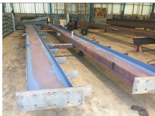
Image showing completed rafter being prepared for paint.
